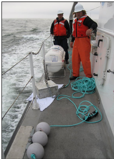
Figure 2-4. Rigging system used to deploy the marine acoustic receiver off of the mouth of the Eel River.
