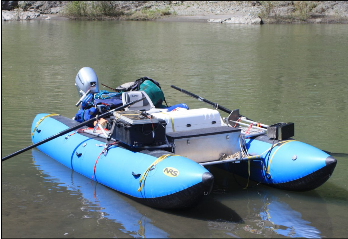
Figure 2-1. Custom motorized whitewater cataraft used for mobile sonar survey in the spring. The DIDSON sonar camera and mounting arm (stowed for rapids) is visible to the right of the photo on the left tube of the boat.
